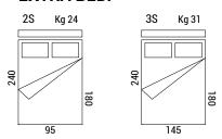
Fire retardant or standard polyurethane mattress, with three-fold mechanism, h 8 cm, covered with antiallergic polyester lining. High-resistance steel electrowelded mechanism
